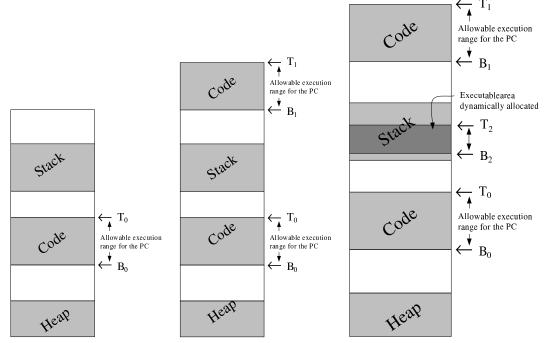
A program normally contains three segments that can be distinguished: heap, code, and stack. We expect the PC to remain in the area between the  $B_0$  and  $T_0$  markers.
