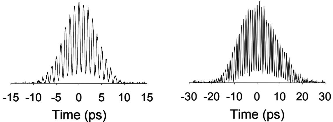
Fig. 1 Intensity cross correlation measurements of the output of 100 GHz output channel spacing (left) and 40 GHz output channel spacing (right) AWG devices both with 1 THz FSR.
