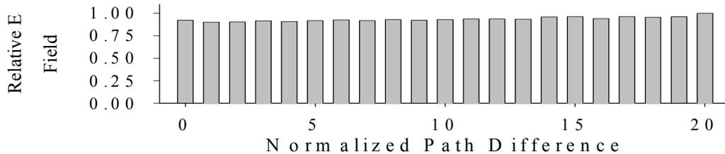
Fig. 2 Measured electric field amplitude in an AWG device designed to have a flat-topped output temporal intensity profile.
