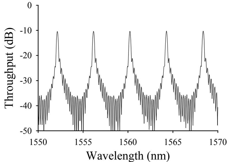
Fig. 3 Measured power spectra from an AWG device with 500 GHz FSR and waveguide losses engineered to generate a flat-topped output temporal intensity profile.
