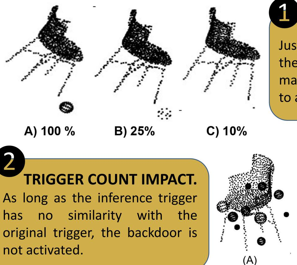
**TRIGGER SIZE IMPACT.** Just a subset of the points of the inference trigger have to match with the original trigger to activate backdoor.
