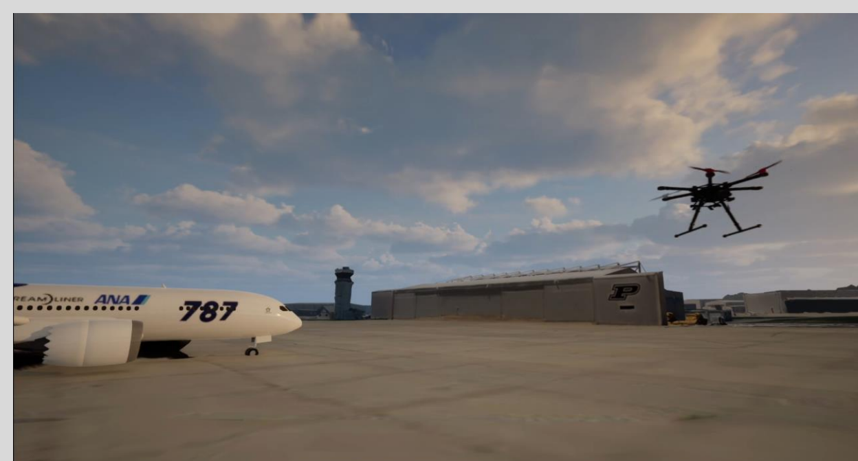
UAV control through AirSim API library and PX4 Software-In-the-loop (SITL)
