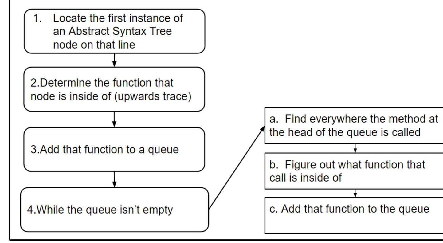
Thus, we working towards developing a control flow analyzer to enumerate the flows that reach the vulnerability.
