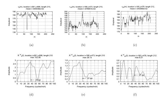
Figure 11. a-c) Runs from actual text Figure 10a, d-f) Corresponding FFT of the processed runs a-c
