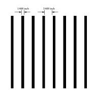
Figure 2. Midtone pattern 25% fill used for banding characterization
