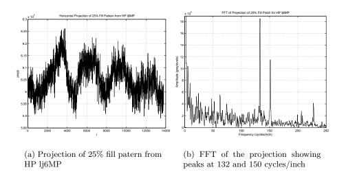
Figure 3. Projection and FFT analysis of 25% fill pattern printed on HP lj6MP
