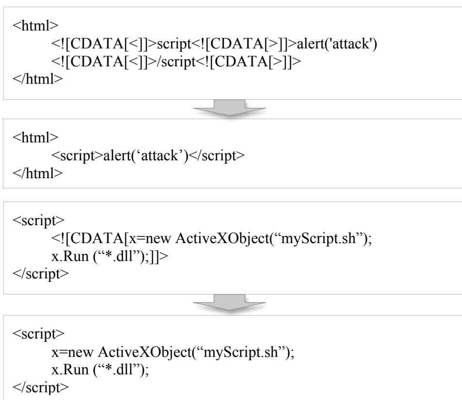
Figure 4.3 Examples of XML Attack by Using CDATA. Box A, B, C, and D from Top to Bottom
