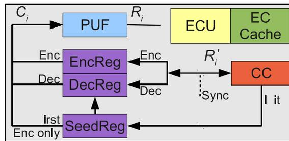
Figure 7.2. Extension components for out-of-order PUF ROKS
