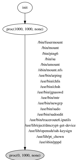
Figure 4.14. Host Attack Graph for a Local Attacker to Install a Rootkit (Ubuntu 8.04 with AppArmor)
