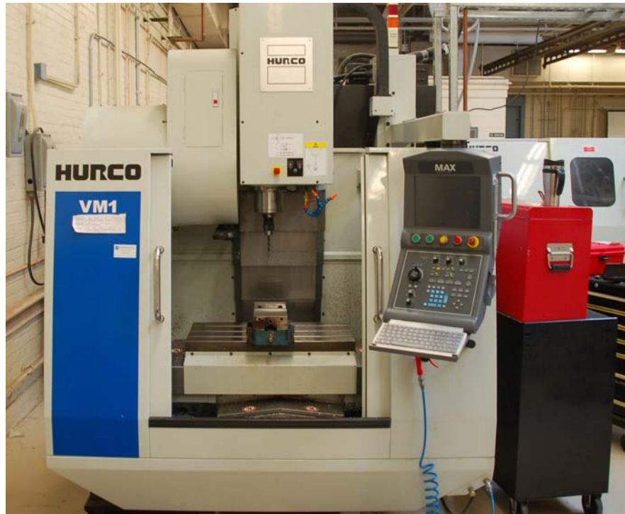
Figure 56 Hurco VM1 vertical machine center used to fabricate the swipe-based form factor devices.
