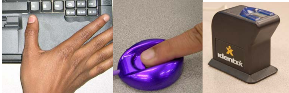
Figure 43 Interaction between thumb and fingerprint swipe sensor produces ulnar deviation (left), Capacitance sensor (middle) and optical fingerprint sensor (right) with finger alignment and guidance impression (Kukula, Elliott, & Duffy, 2007).
