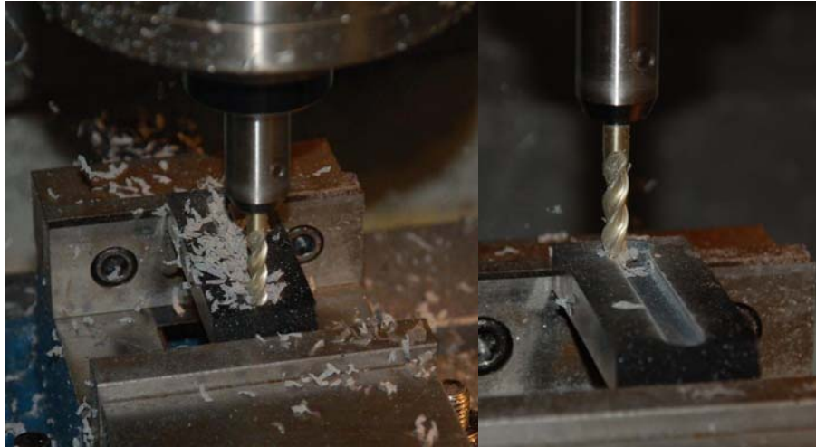
Figure 121 Step 1 of the manufacturing process that created the finger channel.
