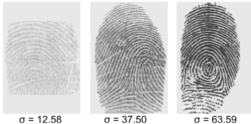
Figure 112 Example fingerprint images from the UPEK sensor showing variations in image contrast values.
