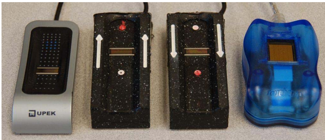
Figure 58 Fingerprint sensors used (from left to right): 1) Eikon swipe sensor, 2) PUSH designed sensor, 3) PULL designed sensor, and 4) TouchChip large area sensor.
