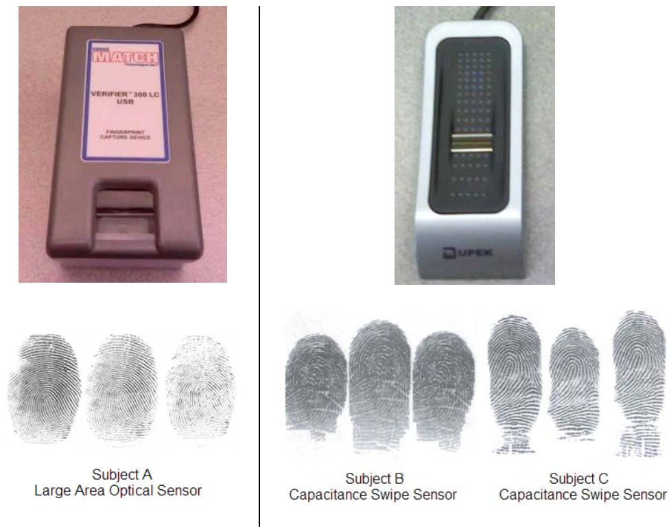
Figure 32 Images captured with different type and size sensors.
