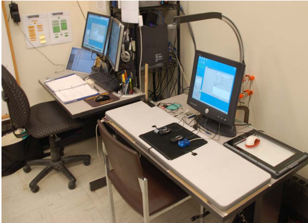
Figure 57 Full view of experimental testing area. The computer on the left is the researcher station. The computer on the right is the data collection computer where participants interacted with the fingerprint sensors.
