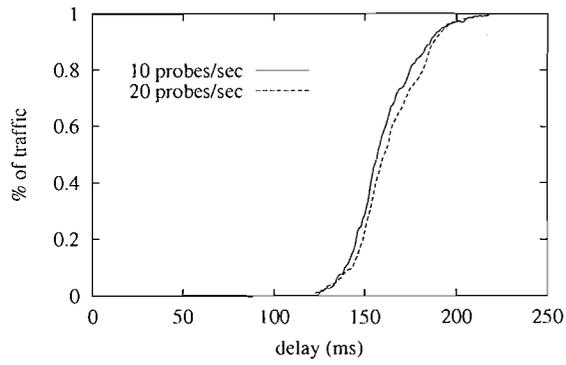
(a) Delay for different probe frequencies
