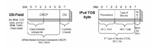
Figure 3: Differentiated Services Code Points redefine the IPv4 TOS byte [QoS99d]
