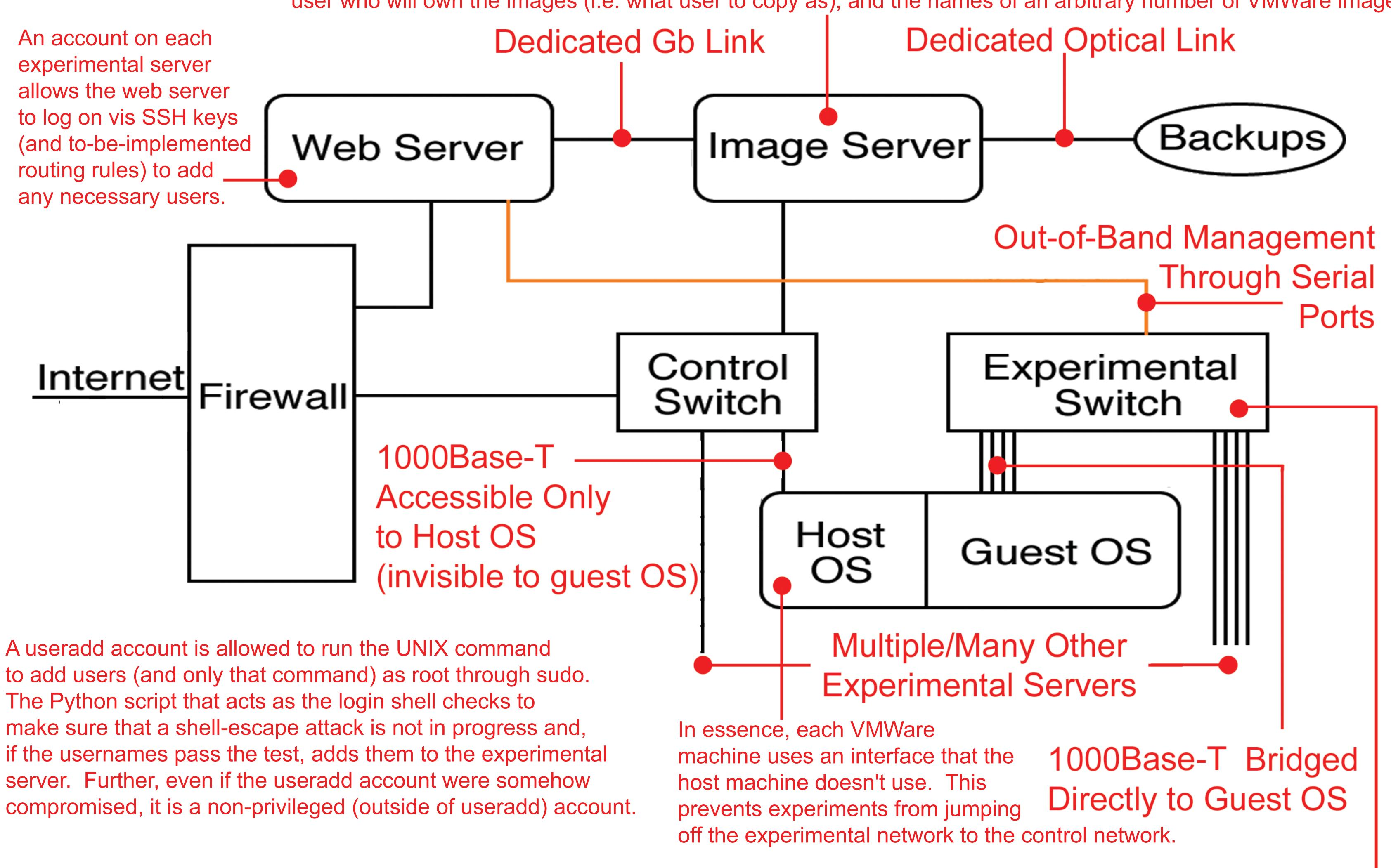
ReAssure utilizes VLANs which are configured on the fly over a serial interface by a handful of custom python library commands. The VLANs offer a very secure logical network which allows experiments to be run in parallel while simultaneously preventing interference between them. The VLANs themselves are controlled by a Cisco 4948 switch that runs Cat IOS 12.2 and offers a switching fabric speed of 96-Gbps.
