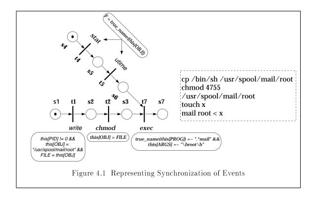
The circles in Figure 4.1 represent system states and the thick bars the transitions. s1 and s4 are the initial states of the CPA, and s7 is its final state. A CPA requires the specification of  $\geq 1$  initial states and exactly one final state. A start state must have no arcs incident on it, and a final state must have no arcs emanating from it. At the start of a match, a *token* is placed in each initial state.
