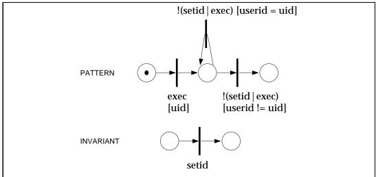
Figure 4.4 A Simlified Pattern to Detect Unauthorized Transitions to Root
