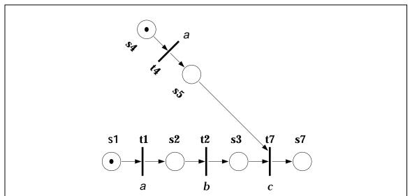
Figure 4.2 Simulation of a Pattern That Does Not Use Guard Expressions or Token Local Variables
