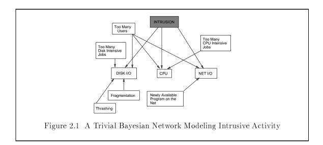
Each box represents a binary random variable with values representing either its normal or abnormal condition. If we can observe the values of some of these variables, we can use Bayesian network calculus to determine P(Intrusion|Evidence). However, in general it is not trivial to determine the *a priori* probability values of the root nodes and the link matrices for each directed arc. For a good introduction to Bayesian Networks see the article by Charniak [Cha91].
