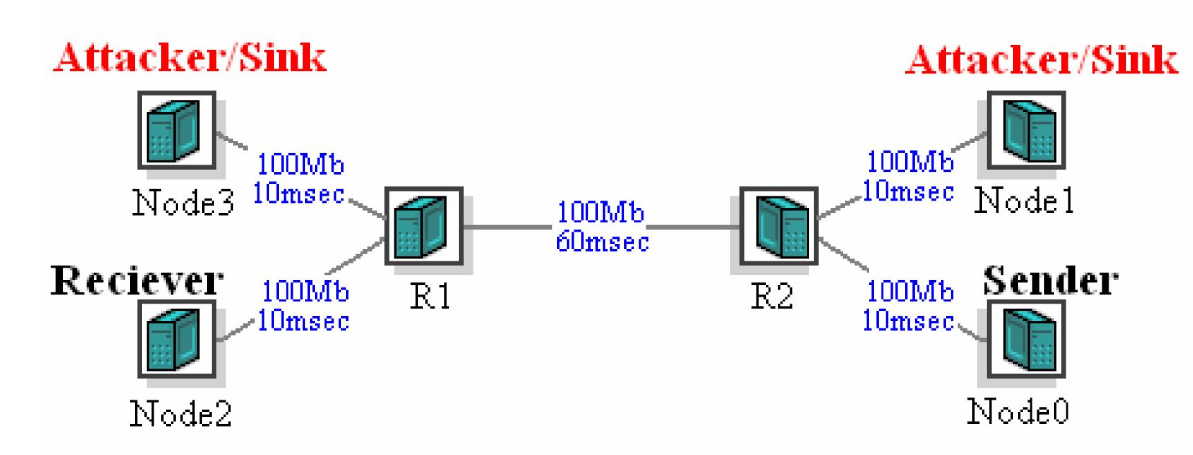
Simple topology for simulating and emulating a TCP-targeted low-rate attack. The attacker sends short pulses at a fixed frequency to exploit the TCP congestion control mechanism.
