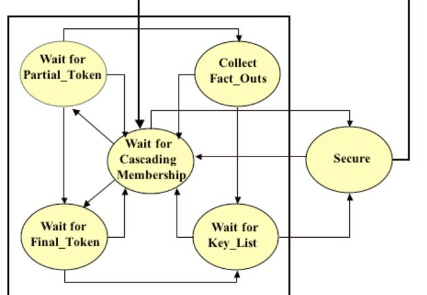
A process can crash/disconnect in any state. The network can partition/merge in any state.
