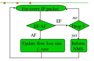
Periodically, with time period t, send the loss rates of all flows with loss rates within a fraction k of the flow with the highest loss rate.
