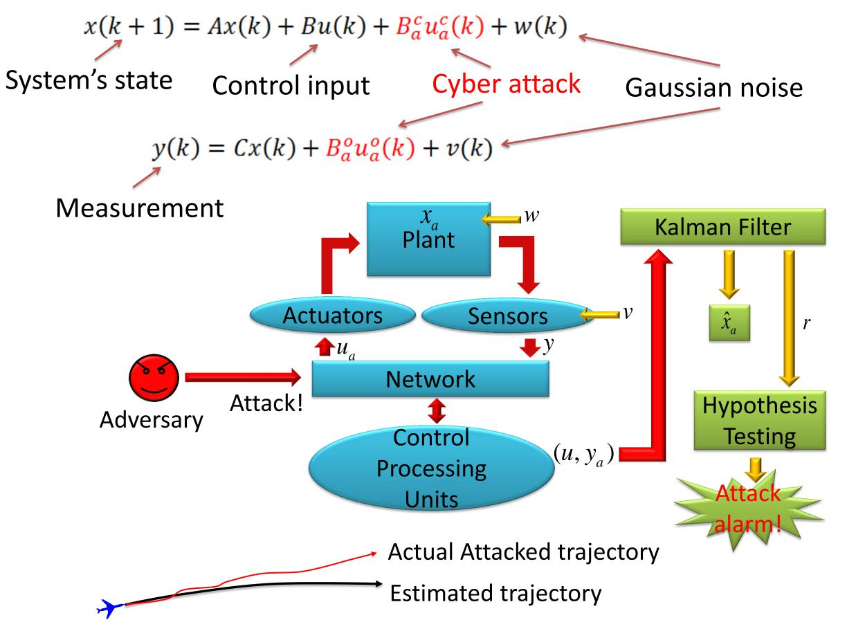
→ <u>Stealthy cyber attack</u>: cause large estimation error without being detected by the monitoring system.
